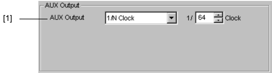
Figure 7.11.6.3-1 AUX Output Setting (When 1/N Clock Is Selected)
